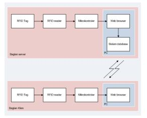
Figure 5. Diagram block of alarm system and medical records.
