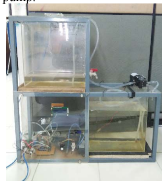
Fig. 2. Experimental set up of water tank system
