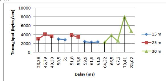
Figure 9. Throughput and delay testing chart with 1 user
