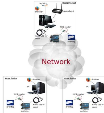
Figure 4. System diagram block
