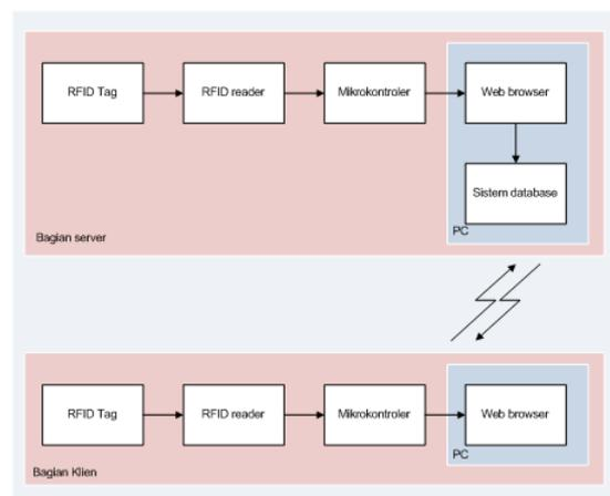
Figure 5. Diagram block of alarm system and medical records.
