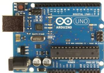
Figure 3. Arduino Uno module
